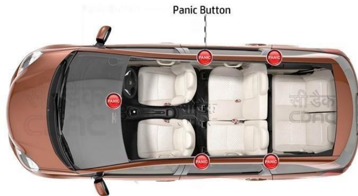
Fig: Position of panic buttons in six/seven seater vehicle
