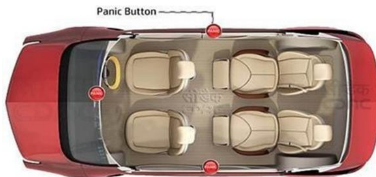
Fig: Panic buttons positions in four seater vehicle
